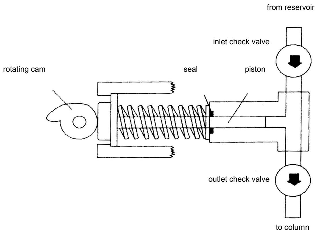
**FIGURE 7.2** A typical single piston HPLC pump (from Ewing, Analytical Instrumentation Handbook, Dekker)
