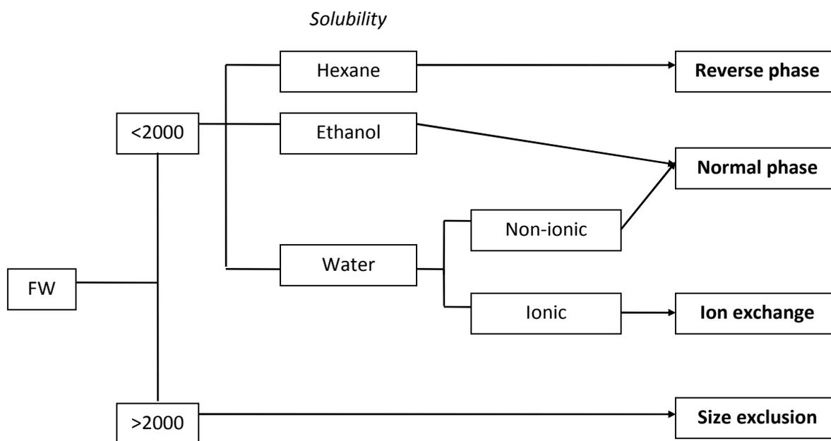
**FIGURE 7.8** Flow diagram for selection of HPLC stationary phase
