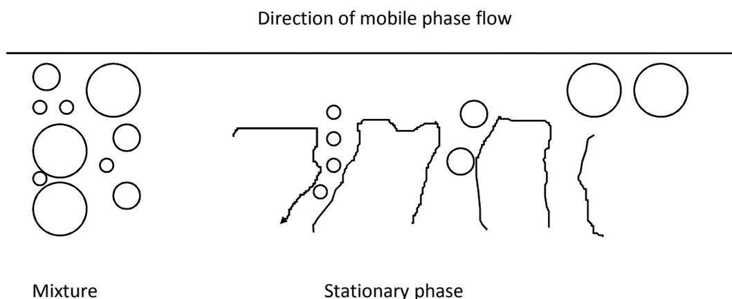
**FIGURE 7.6** Separation mechanism in size exclusion chromatography
