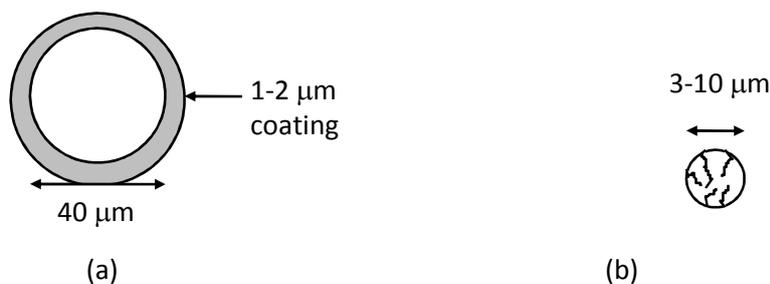
**FIGURE 7.3** HPLC column packing materials (a) pellicular (b) microparticle (not to scale)
