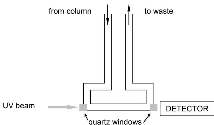
**FIGURE 7.4** Schematic diagram of a flow-through UV detector cell
