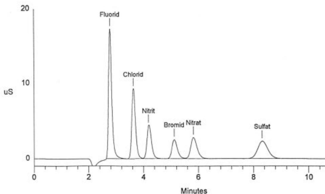
FIGURE 7.5 Ion chromatogram for a mixture of anions (from [www.bayer.com](http://www.bayer.com))
